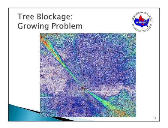
Here is the ZDR image from KHPX, showing the two regions of beam blockage as wedges of higher ZDR.
