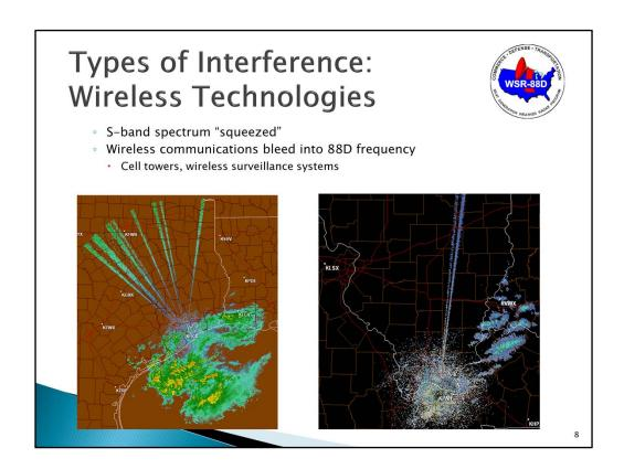
The S-band is becoming increasingly crowded, with many types of systems competing for the same frequencies. Interference from cell phone towers is one of the most common types of interference seen on the WSR-88D, but can be caused by other wireless emitters.
