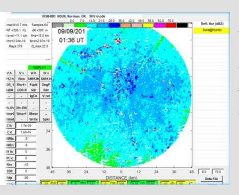
WSR-88D KOUN (Norman, OK). Ground clutter filter is on.
